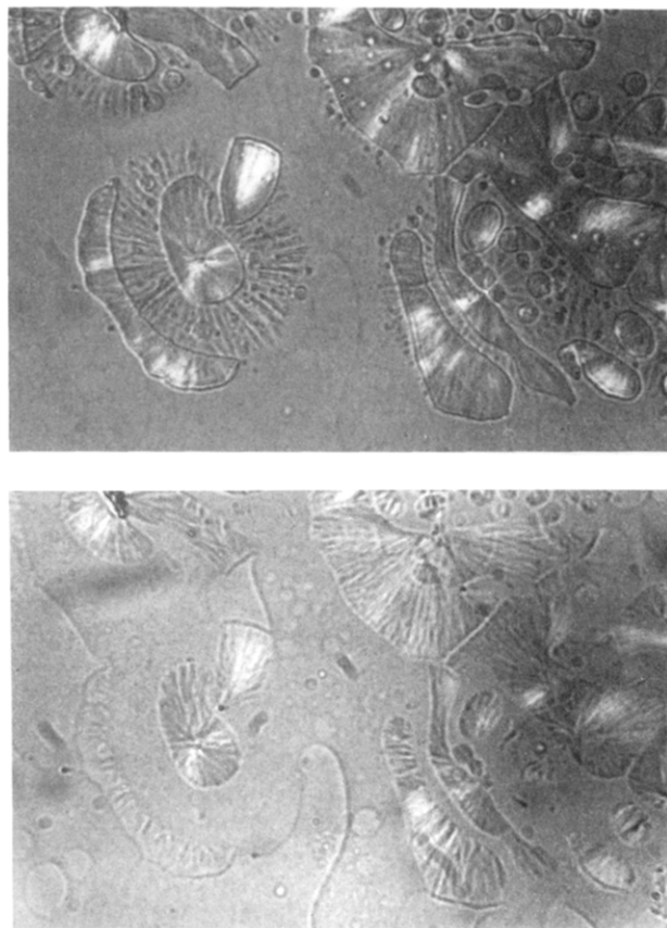
Figure 5. Optical micrographs of a 30/70 it-PP/it-P1B blend at various temperatures during heating from 145 to 180 °C at a rate of 5 °C/min. This sample was isothermally crystallized at 145 °C for 210 min after residing at 180 °C for 5 h (same region as on Figures 3 and 4): (a) 155, (b) 165, (c) 172, and (d) 173 °C (same magnification as in Figure 1a).
